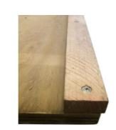
Add two guide rails of 45mm x 20mm or similar down either side of the base table ensuring CLEVA POD® fits snuggly between guide rails.
