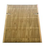
Cut a base table from 18mm plywood or similar: 1450mm x 1200mm.
