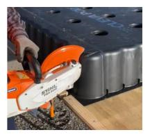
The Saw cuts cleanly through the CLEVA POD<sup>®</sup> and passes down through the cutting slots.
