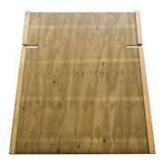
Cut a base table from 18mm plywood or similar: 1450mm x 1200mm.
