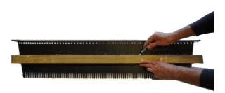
If a cut down baffle is required for a shortened pod, measure 100mm up from the base of the CLEVA COMB<sup>™</sup> teeth.
