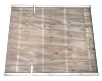
Measure 1020mm along both edges and cut two 30mm wide x 150mm long cutting slots into the cutting table.
