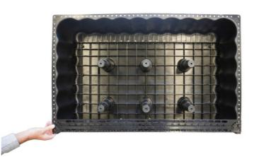
Place a CLEVA COMB™ across the exposed face of the CLEVA POD<sup>®</sup>, push the CLEVA COMB<sup>™</sup> firmly down into the grid securing the CLEVA COMB™ teeth into the pods structural grid and connect to pre-drilled base flange using the CLEVA PLUG™s.
