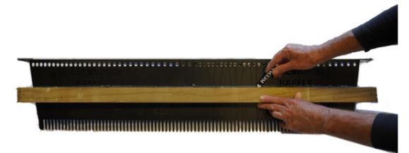
If a cut down baffle is required for a shortened pod, measure 100mm up from the base of the CLEVA COMB™ teeth.
