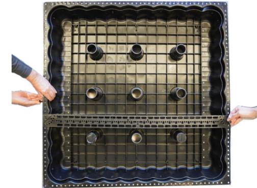
Push the CLEVA COMB™ firmly down into the grid securing the CLEVA COMB™ teeth into the CLEVA POD® structural grid and connect into the pre-drilled base flange using the CLEVA PLUG™s.
